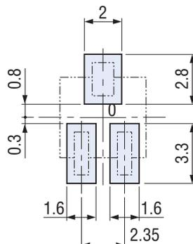
Note) The zero point is the center of mounting.
